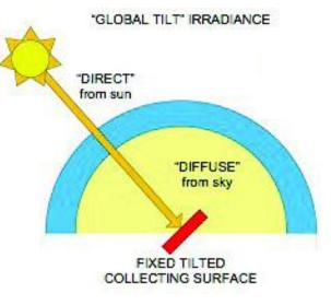
**Global horizontal irradiance (GHI)** is the sum of the projected DNI on a horizontal surface and of diffuse horizontal irradiance
