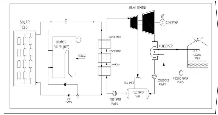
The combination of these two technologies benefits from increased overall efficiency of the power plant, reduced number of shutdowns of the turbine and reduced investment per unit of power generated compared to CSP with molten salts heat storage, for example
