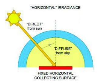
**Direct normal irradiance (DNI)** is the fraction of the downward flux directly emanating from the sun disk that is incident on a plane normal (i.e., perpendicular) to the sunbeams, and that has not undergone any extinction in the atmosphere NA.2012.A.002.0
