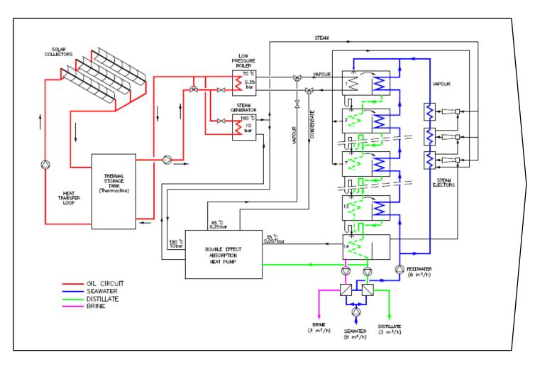
Schematic diagram of the solar MED system installed at PSA
