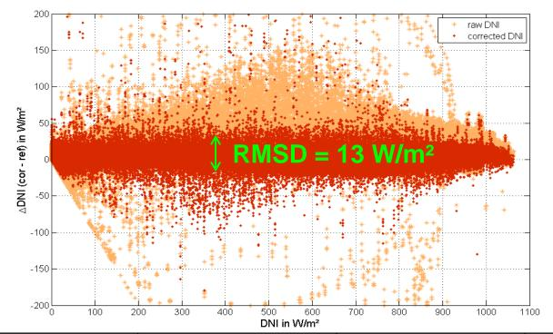
derived from data comparison of 23 RSIs with High-Precision Instruments within the course of a whole year
