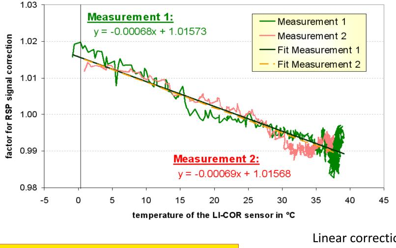
$$CF_{temp} = (1 - 0.0007 \cdot (T_{LI-COR} - 25^{\circ}C))$$
