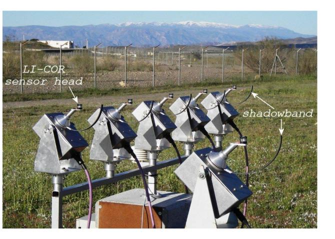
Calibration of the RSIs: for example by German Aerospace Center (DLR) during 2 months against High-Precision instruments on Plataforma Solar de Almería *(recommended frequency:*
