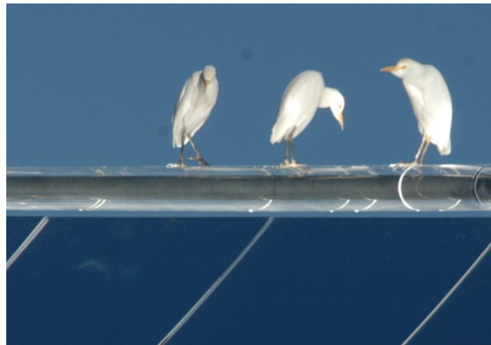
Figure 2.7 - Receivers with black, sputter coated inner stainless steel pipe and evacuated glass envelope, reducing thermal losses to a minimum.
