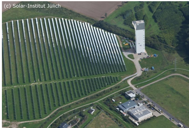
Figure 2.17 - Solar Tower Jülich with volumetric air receiver technology (Source: SIJ).
