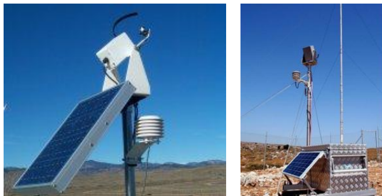
Figure 12.4 - Examples of RSI stations. Left: Irradiance, Inc. right: CSP Services GmbH.
