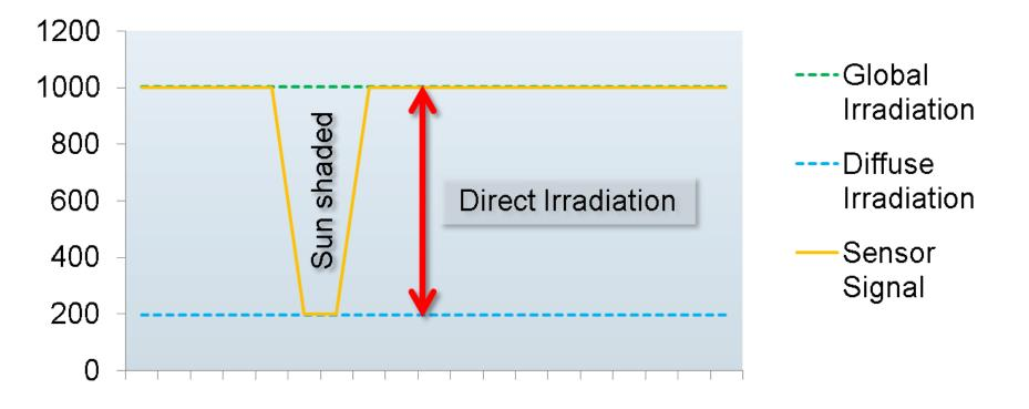
Simplified sensor signal during shadow band rotation: once per minute, rotation lasts about 1.5 seconds
