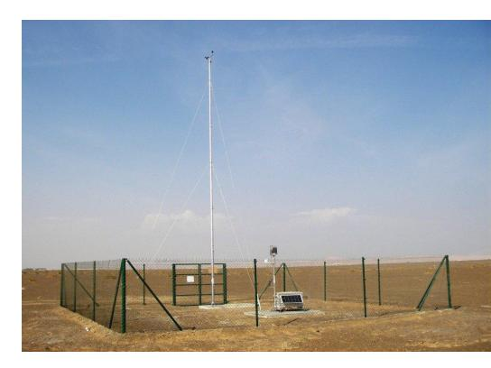
MDI instrument control box containing PV panel, battery, datalogger and communication modem
