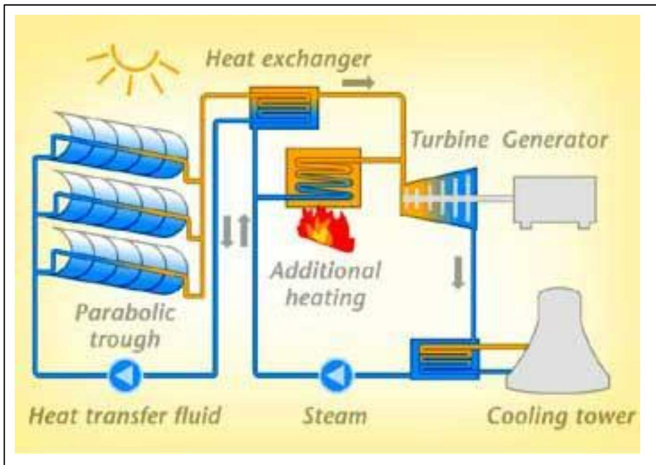
The concept of backup is simply explained in the following diagram
