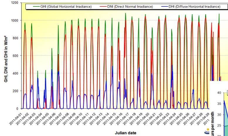
MHP Weather Station, Plataforma Solar de Almería, Spain - April 2011
