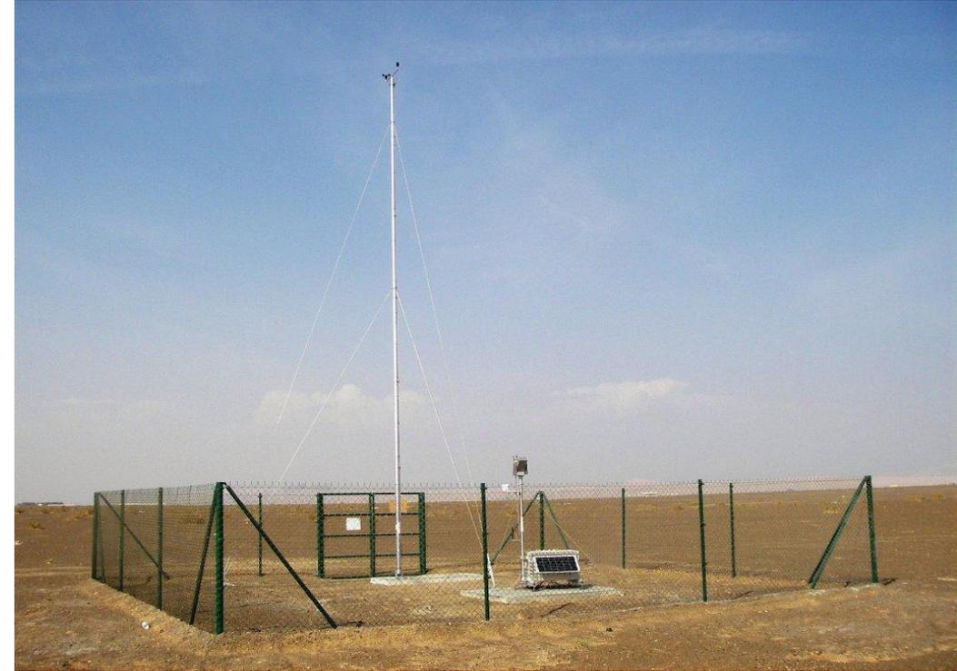
MDI instrument control box containing PV panel, battery, datalogger and communication modem
